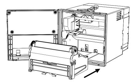
6th Push recording paper cartridge into KRN100 until click sound. Close front cover of KRN100.
