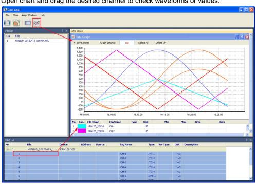
3rd Open chart and drag the desired channel to check waveforms or values.
