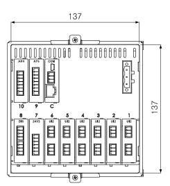
X Back side dimension is with installed I/O cards to every slot.
