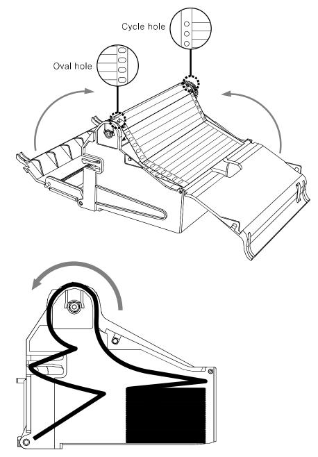
5th Put recording paper's holes (circle, oval) at recording paper holder and close new recording paper storage cover and finished recording paper storage cover.
