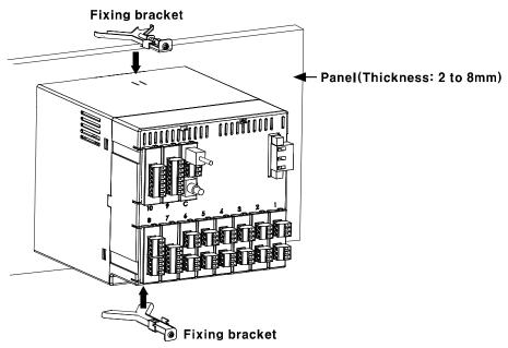
2nd Tighten fixing brackets on upper/lower parts to fix on the panel with phillips screwdriver (+). (Torque: 0.4N•m)
