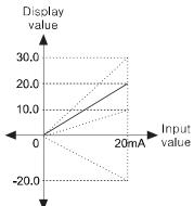
Set Low Scale (Lower limit scale value) = 20.0, High Scale (Upper limit scale value) = -20.0.
