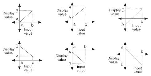
You can change display value about min./max. input value of measuring value.
