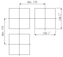
X Use panel which is 2 to 8mm thickness.
