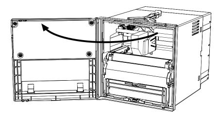
2nd Push down recording paper cassette lever placed at below recording paper cassette, recording paper cassette is removed from KRN100.
