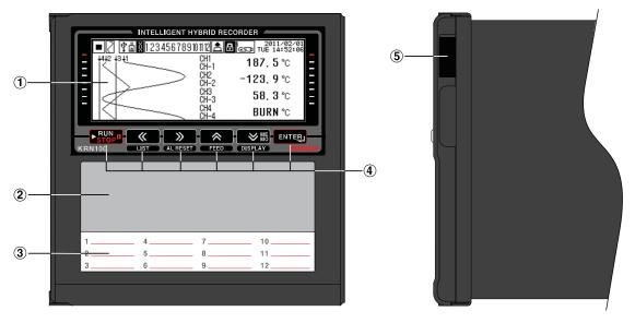
Display part: Displays measurement values as trend graph, bar graph, or digital number (1/8/12 channel).
